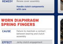
Renew cover assembly, check release mechanism (including self adjustment) for correct operation. Observe correct adjustment frequency and procedure
